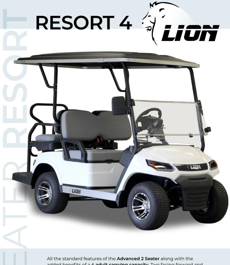
All the standard features of the **Advanced 2 Seater** along with the added benefits of a **4 adult carrying capacity**. Two facing forward and two rear facing seats with the back seat capability of folding down into a handy tray. A full length roof is also fitted as standard equipment along with safety hold rails for rear passengers. Seat belts fitted to all seats.
